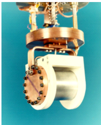
Fig. 1: Shows a standard vapour pressure sample set up used to study Helium films in porous media at 300mK in an adsorption cryostat.
