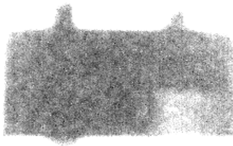
Fig. 1: Neutron image of the mixing chamber of a DR, showing the difference in neutron transmission through the highly absorbing 3 He rich phase and the weakly absorbing 3 He poor phase.
