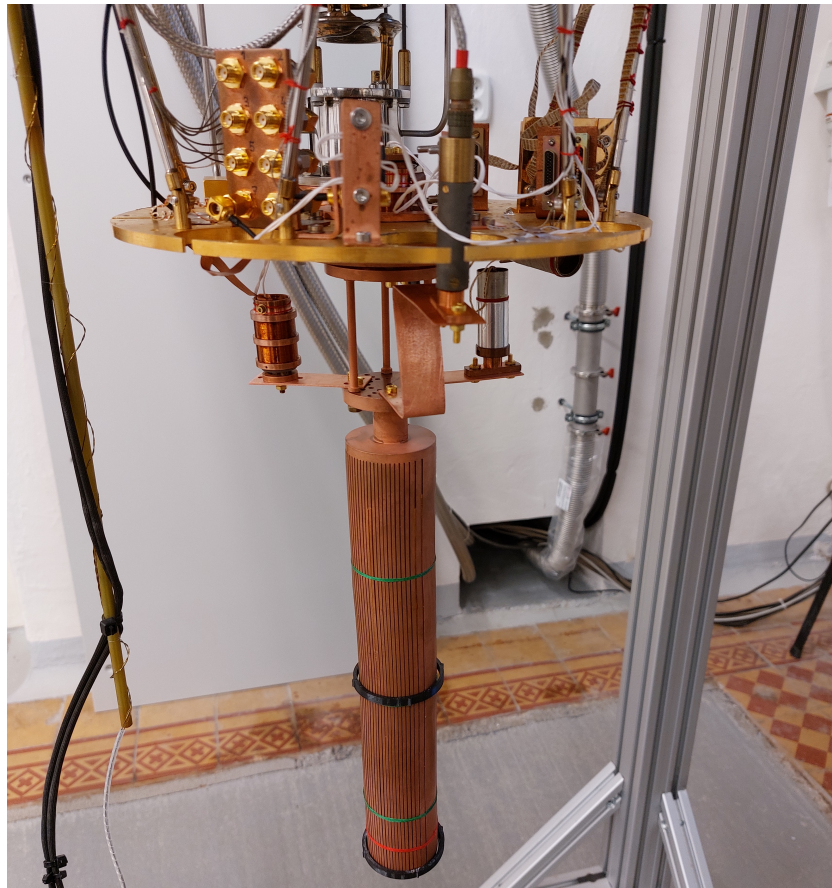
Figure 1: Photograph of the ”plug-in & cool” copper nuclear demagnetization stage .
